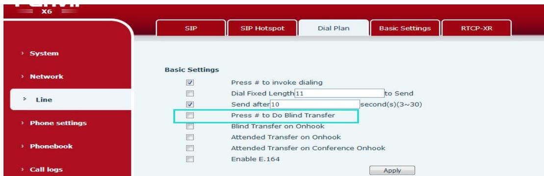
Select **Press # to Do Blind Transfer**, enter the number on the transfer dialing interface, and press # to perform blind transfer. If you do not select this option, the phone does not perform blind transfer after you press #.
