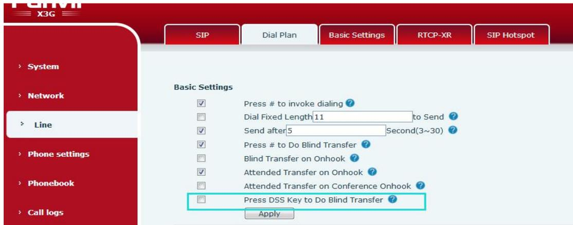
After adding a number to the memory key and pressing the transfer key, you can press this key to transfer the call to the third party.
