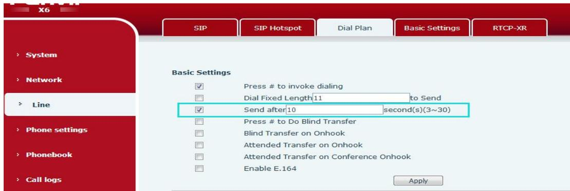
Configure the timeout interval, in seconds. For example, when the timeout is set to 10 seconds, if you do not enter the second digit 10 seconds after the first digit, the phone considers that you have completed dialing and delivers the entered digit.
