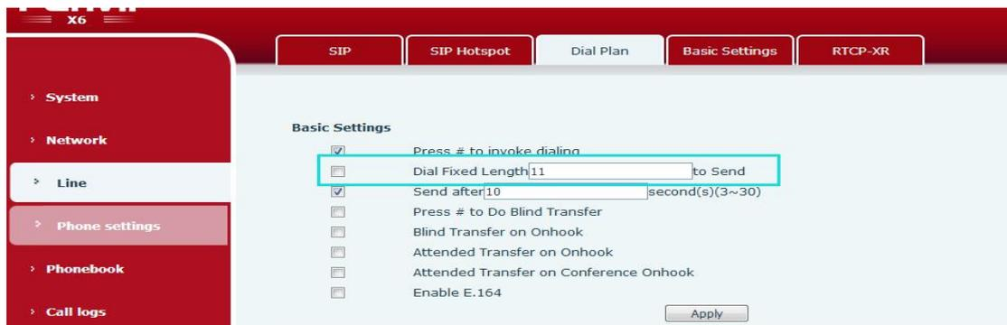
Configure the phone to collect digits with a fixed length. For example, if the fixed length is set to 11, the phone automatically dials out when 11 digits are entered.
